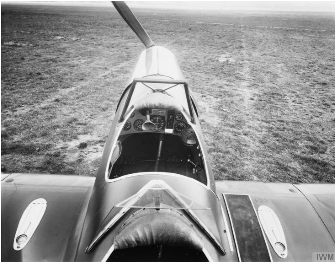
The forward cockpit. The speaking tube is visible- the way student and instructor communicated. This aircraft has more instruments than the Tiger Moth.
