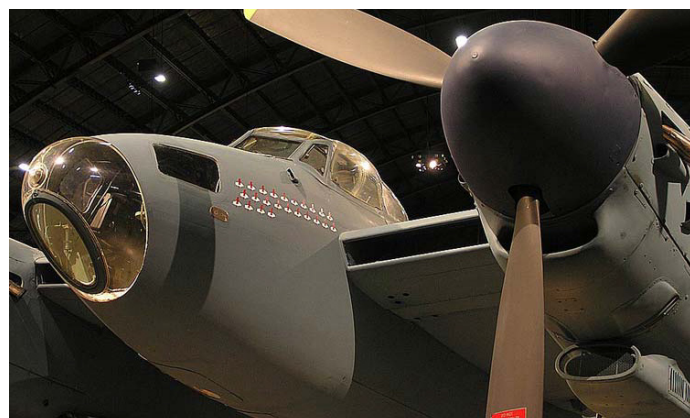
Radiators were mounted behind the rectangular openings in the wing root.
