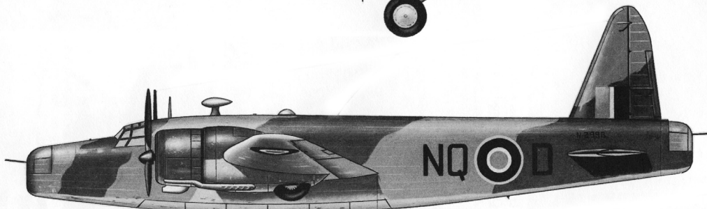
Vickers Wellington transport of No. 24 Squadron, Royal Air Force, with false nose and tail turrets painted on to make ship resemble standard Wellington bomber.
