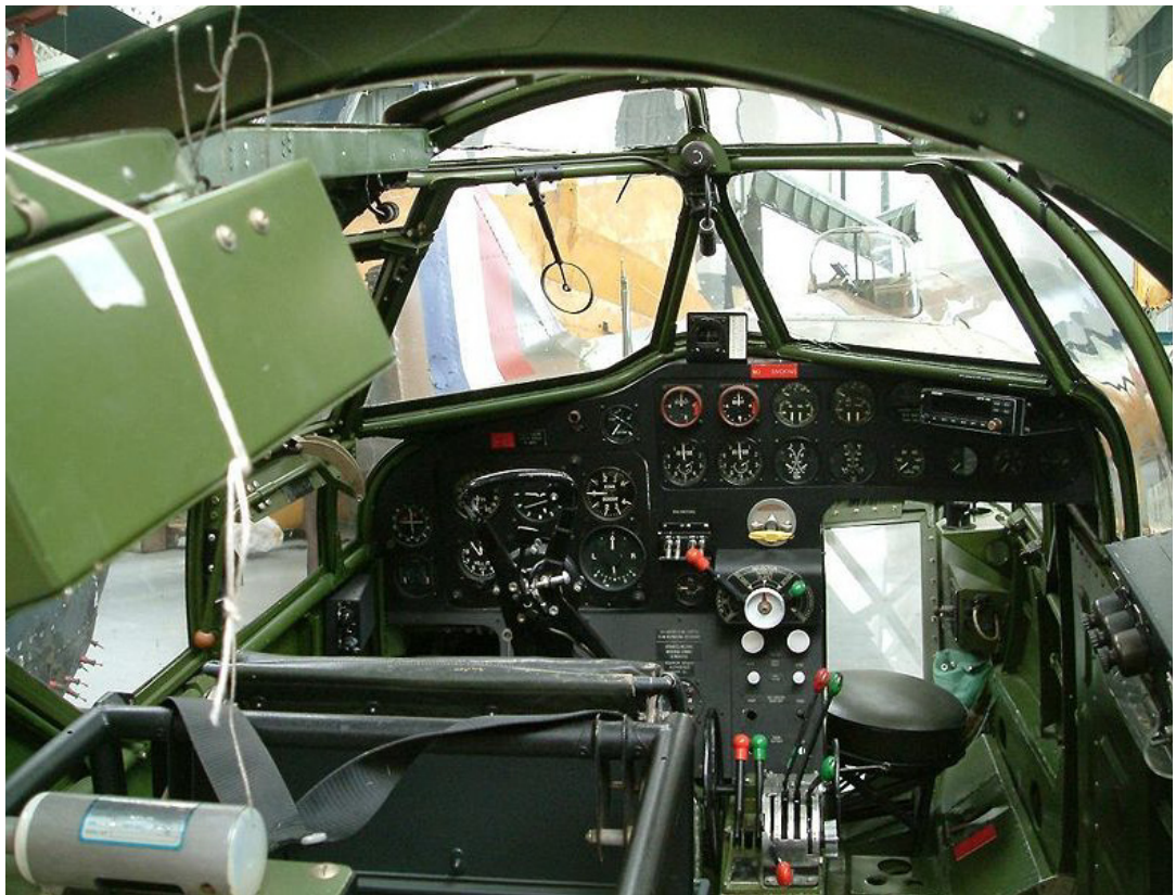
The Blenheim Mk IV cockpit. The navigator position was in the nose, in front of the pilot. The ring and bead gunsight for the forward firing guns is visible. The pilot and navigator had to lower themselves in via a hatch above the cockpit, and minor scrapes and cuts were common. The navigator/ bomb aimers position in the Mk I was cramped, with no space for a proper map table. However, the pilot did have excellent visibility.
