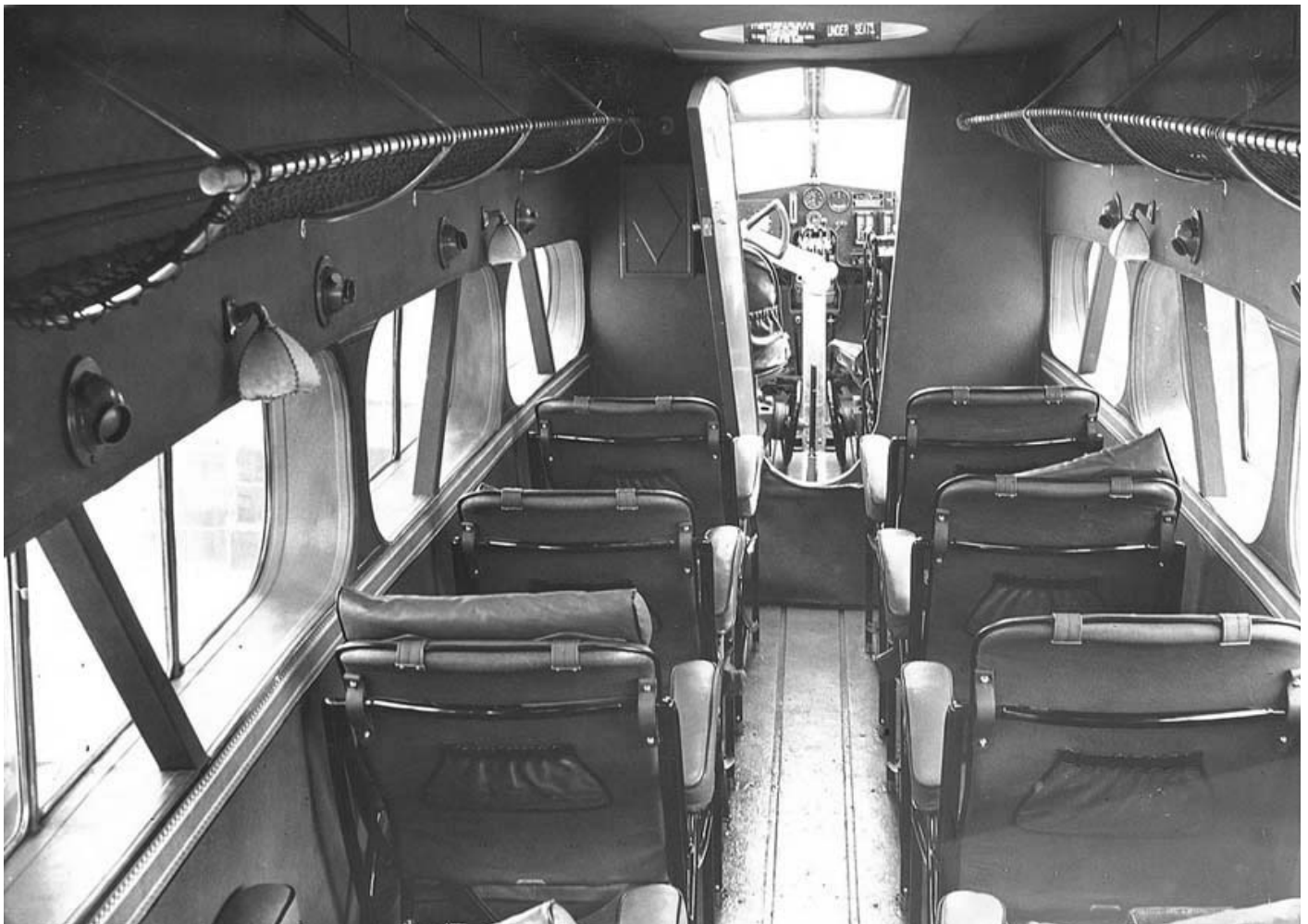
The interior normally held 10 passenger seats, with some aircraft carrying an additional two seats. Two pilots sat in front.
