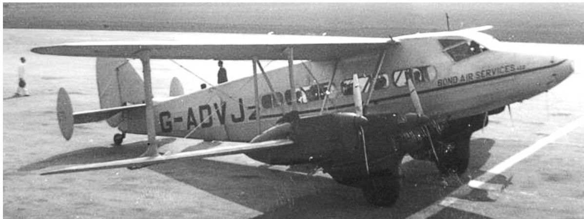
The DH 86B is shown (left) with the extra fins on the tail to improve stability. The 3-view drawing below shows the original DH 86 with a single tail fin.
