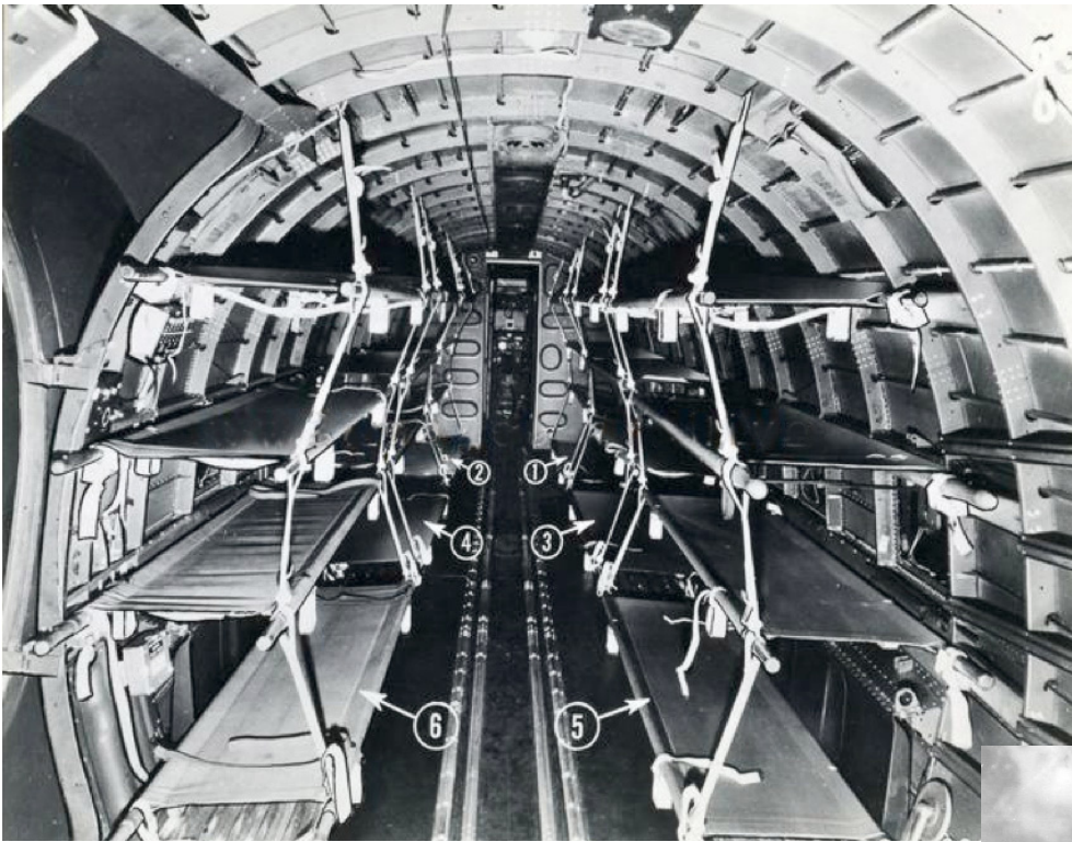
Some C-47s were fitted out as air ambulances. There was space for 18 injured people, stacked three high along the cabin wall.
