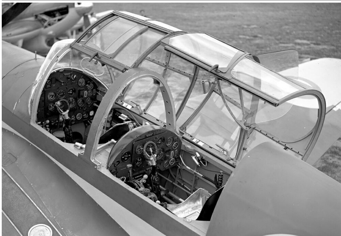
Two views of the Miles Master cockpit. The student sat in front, the instructor in back.
