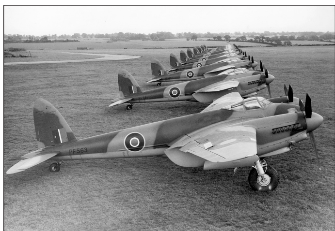
Radiators were mounted behind the rectangular openings in the wing root.
