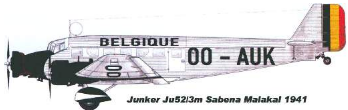
Junkers Ju52- 17 passengers, 138 mph cruise speed, Range: 590 mi (950 km)
