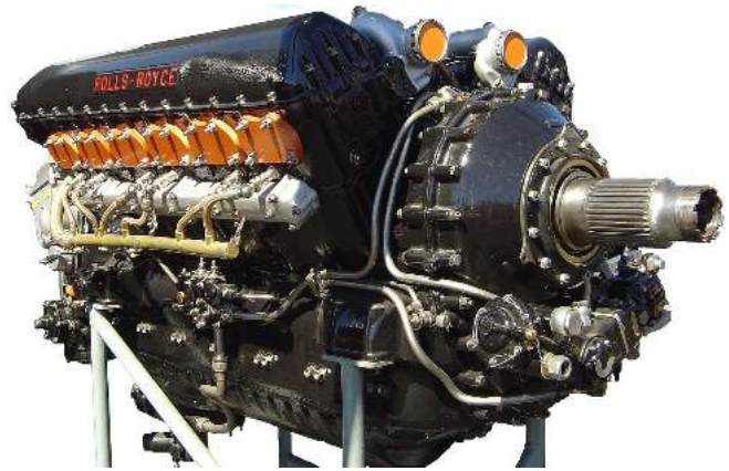
Showing the small frontal area of a V type liquid-cooled engine
