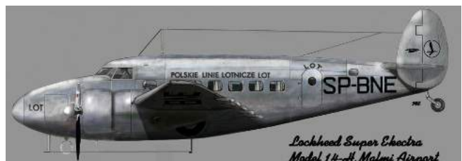
Lockheed L-14 Super Electra: 12 to 14 passengers, 215 mph cruise speed, range 851 mi (1,370 km)
