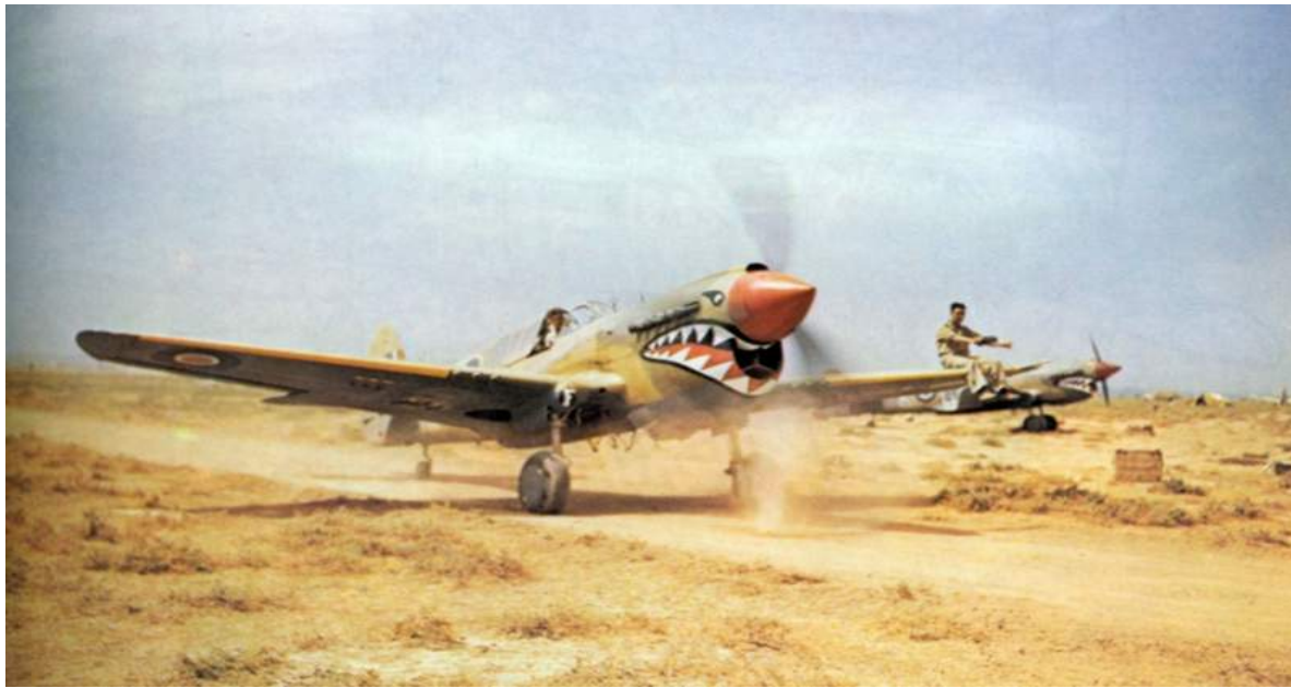
1943: A Kittyhawk Mark III of 112 Squadron, taxiing through scrub at Medenine, Tunisia. The aircraftman sitting on the wing is directing the pilot, whose view ahead is hindered by the aircraft's nose, a common problem for tailwheel aircraft when taxiing.
