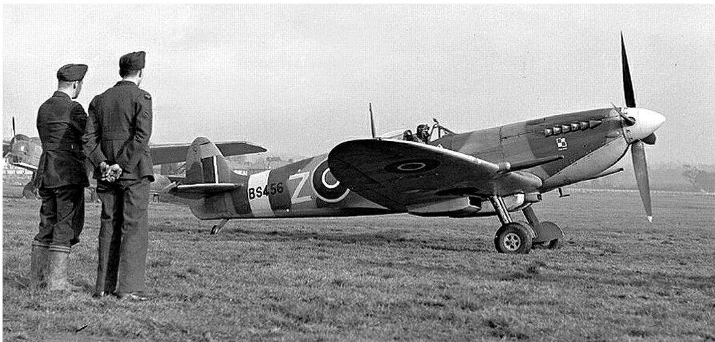
Spitfire of Lt L. Kurylowicz of the 303 (Polish) Squadron. The Spitfire on this and the facing page is a later model version (post-1943) with a larger, more powerful Rolls Royce Griffon engine driving a 4-bladed propeller. Each of these Spitfires carries one Hispano II cannon in each wing, which fired 20mm (0.79") shells. Each gun could be fed 120 rounds.
