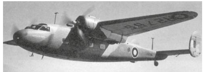
De Havilland DH95 Flamingo, 17 passengers, 204 mph cruise speed, Range: 1,345 mi (2,165 km)
