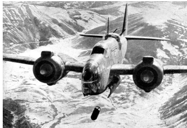
The extremely narrow fuselage created less drag, but bedeviled crews.
