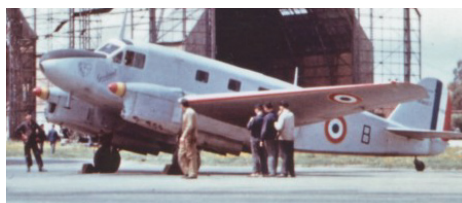
Caudron Goeland French light transport, 6 passengers, gross weight: 3,500 kg (7,716 lb), 2 Renault 220 hp engines, 300 km/h (186 mph) max. speed, Range 1,000 km (620 miles)
